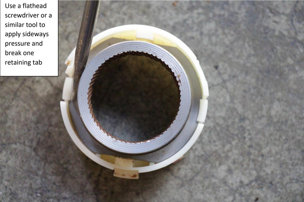
Once a retaining tab is broken, the metal will easily separate from the burr holder
