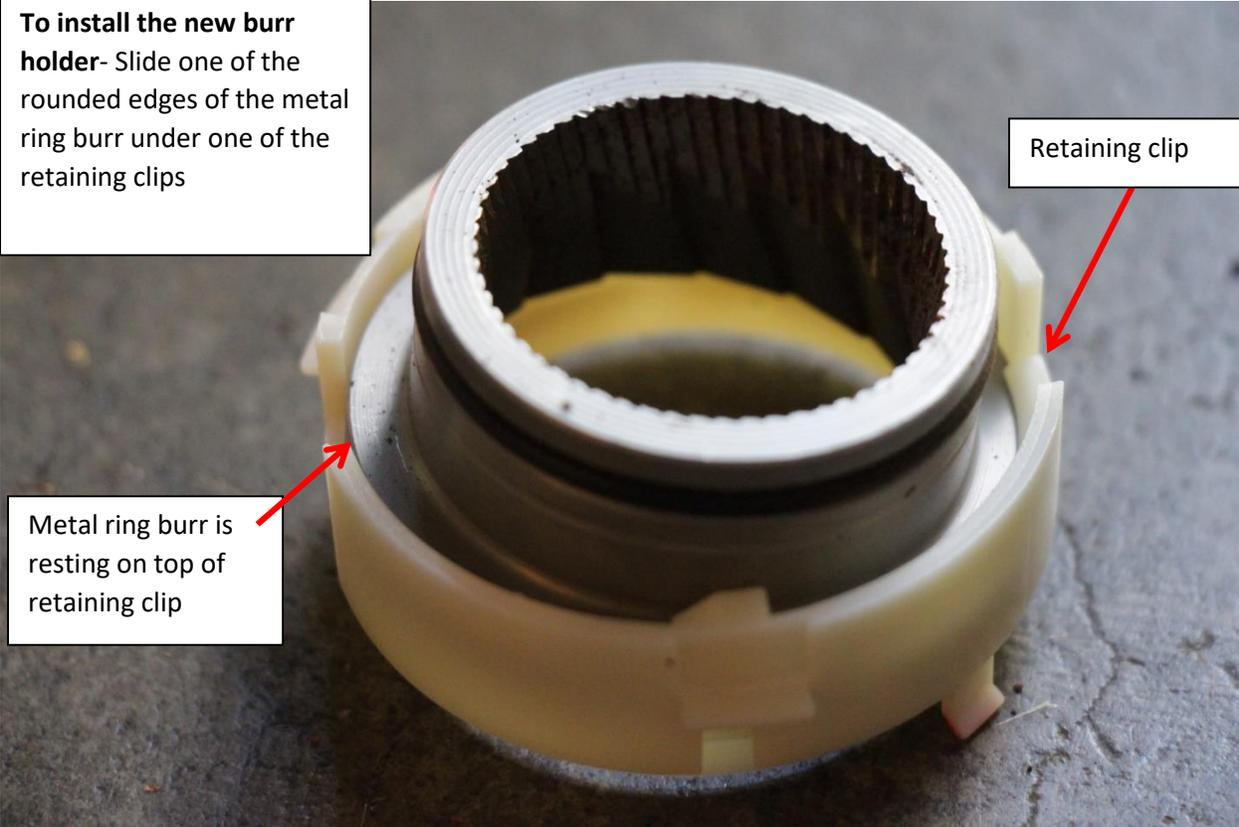
Squeeze the parts together hard to snap the second retaining clip over the metal ring burr
